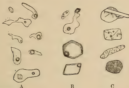
FIG. 7.—CAVITIES IN CRYSTALS, HIGHLY MAGNIFIED. A, LIQUID INCLUSIONS; B, GLASS INCLUSIONS; C, CAVITIES SHOWING THE DEVITRIFICATION OF THE ORIGINAL GLASS BY THE APPEARANCE OF CRYSTALS, ETC., UNTIL IN THE LOWEST FIGURE A STONY OR LITHOID PRODUCT IS FORMED.
